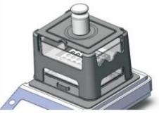
Calibration method: Use a 1000g weight to calibrate.
