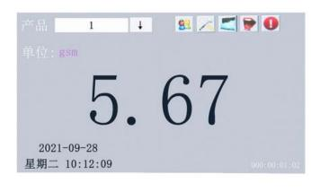
Moisture value upper and lower limit warning function. Once the limit is exceeded, the instrument will automatically change the value into a red letter warning display. 7-inch color touch screen.
