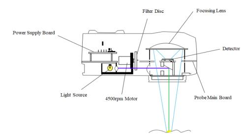
Online moisture analyzer installs a precision infrared filter on the wheel, so that the pulses of reference light and measurement light can alternately pass through the filter. First, the reference light is projected on the sample, and then the measurement light is also projected on the sample. These two sequential light energy pulses will be reflected back to the detector and converted into two
