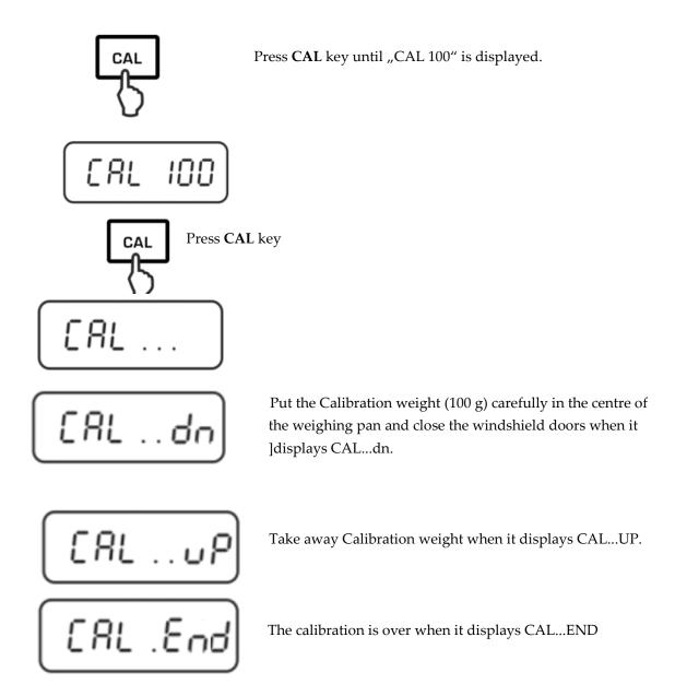
After successful Calibration the balance automatically returns to weighing mode.
