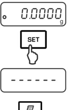
In weighing mode press first the SET key
