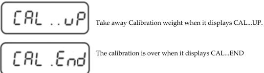
After successful Calibration the balance automatically returns to weighing mode.
