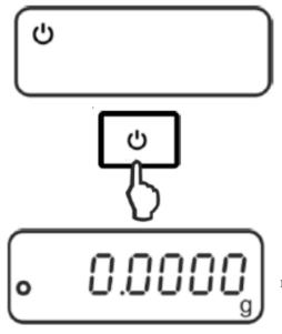
As soon as the balance is supplied with energy, the indicator  $[{}^{\mbox{0}}]$  is displayed.
