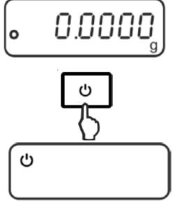
Press **ON/OFF** key, the display disappears and the indicator  $[{}^{\mbox{\iff}}]$  is displayed.
